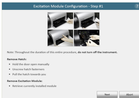
Figure 88. Custom Fluorescence Excitation Module configuration procedure.
