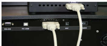
Figure 114. Cable connection of injector system to GloMax® Discover Instrument.
