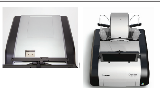
Figure 109. Positioning the Injector System on top of the GloMax® Discover System.
