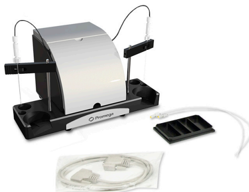
Figure 105. GloMax® Dual Injector System with Pump Station and accessories. Shown assembled here are the Injector System Console with Vertical Support Rods, Inlet Tubing Assembly and Inlet Tube Holder. The DB-15 Data Cable, Waste Collection Tray and Outlet Tubing Assembly are also shown.
