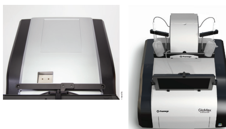
Figure 106. Positioning the Injector System on top of the GloMax® Explorer System.
