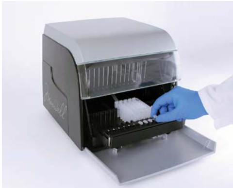
Figure 48. Post-run actions. Close the elution tube caps (A), then remove the deck tray from the instrument (B).
