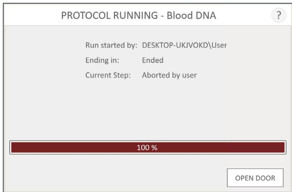
Figure 50. 'Protocol Running' screen after abort by the user. If a method is aborted by the user, the 'Protocol Running' screen will display a progress bar of 100%, and Current Step is shown as Aborted by user. After a method is aborted, press the Open Door button.
