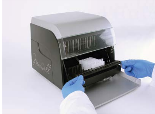
Figure 48. Post-run actions. Close the elution tube caps (A), then remove the deck tray from the instrument (B).
