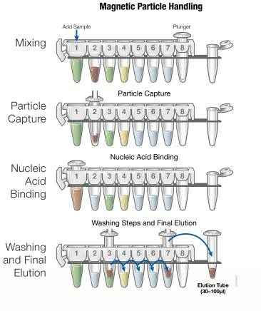
A magnetic bar assembly covered by a plastic sheath (plunger), moves the paramagnetic particles from well to well eliminating clogs, breakdowns and cross contamination.
