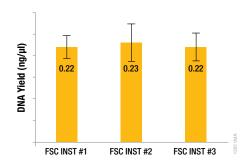
DNA was extracted from 1 $\mu$ l of blood dried on a cotton swab using the Maxwell® FSC DNA IQ<sup>TM</sup> Casework Extraction Kit and the Maxwell® FSC Instrument (N = 3).
