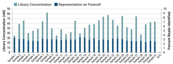
Thirty-two libraries were quantified using the PowerSeq<sup>™</sup> Quant MS System. The resulting values were used to normalize loading of samples into a final sequencing pool. The percent of reads identified for each sample from the total reads generated in the sequencing run demonstrates how evenly each sample was represented on the MiSeq<sup>®</sup> flowcell in relation to all libraries sequenced.
