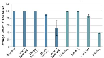
2800M Control DNA was amplified in triplicate in the presence of increasing amounts of common inhibitors. A pool of 32 samples amplified in the presence of tannic acid or  ${\rm CaCl_2\ was\ sequenced\ simultaneously\ using\ MiSeq^{\it @}\ Reagent\ Kit\ v3,\ 2\times300\ cycles.}$
